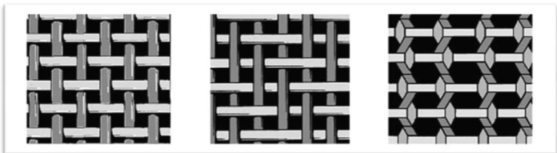
Slika 6. Različite metode tkanja: a) Obično tkanje, b) Keper tkanje, c) Gazno tkanje “Materials and technological development of screen printing in transportation” str. 135.
