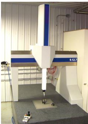
Figure 1: Contact scanner, rigid arm
