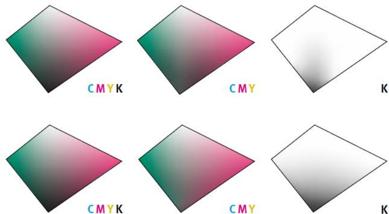
Slika 5 . Široka i uska crna Izvor: Homann, J-P. (2009). Digital Color Management Principles and Strategies for the Standardized Print Production
