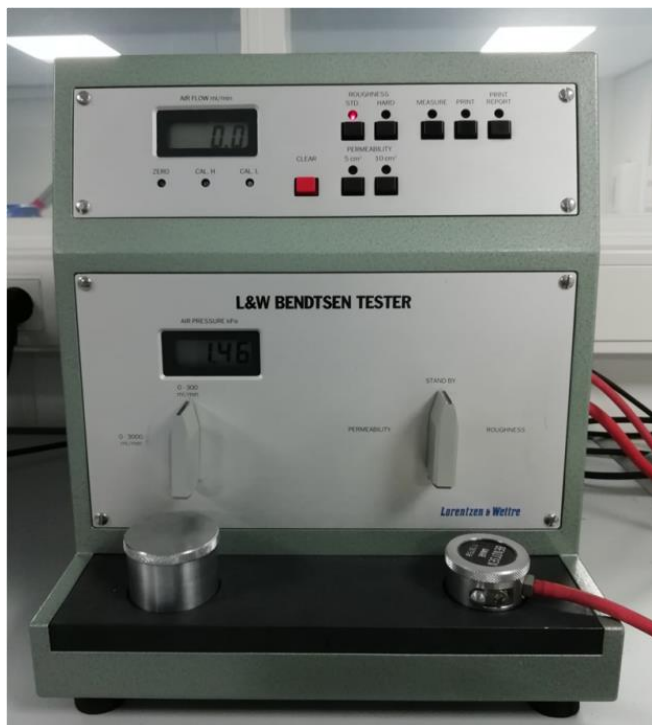
Figure 25 - L&W Bendsten tester
