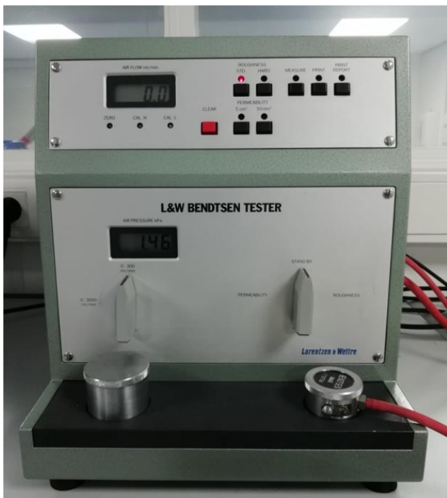
Figure 25 - L&W Bendsten tester
