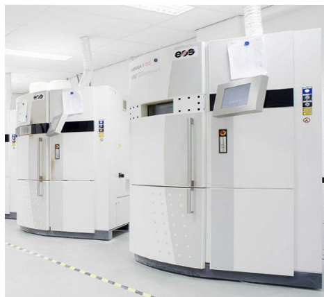
Slika 9. Prikaz SLS printera (Izvor: Redwood, BenSchöffer, Filemont Garret, Brian The 3D Printing Handbook)
