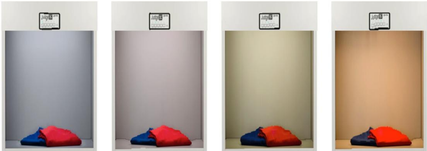
Figure 7. Illuminant metamerism due to the change on different SPD, CCT, CRI [197]
