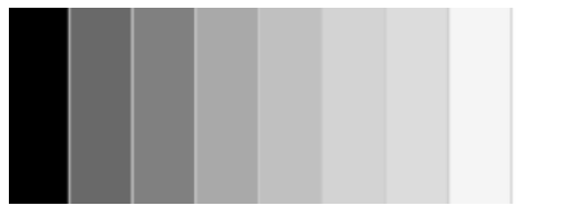
Figure 28. Sample of grey balance field in reproduction printing
