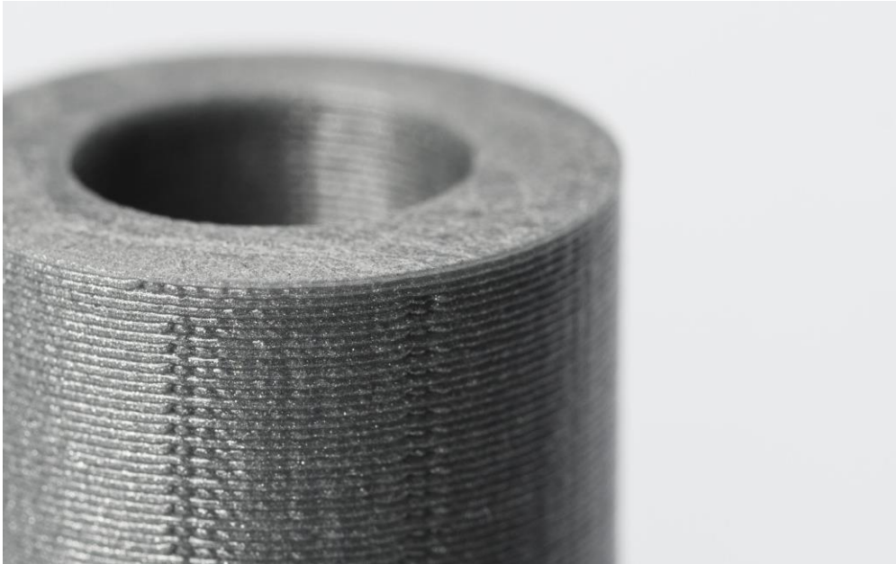
Slika 1.5 – Prikaz slojevitog objekta nakon printa ( https://www.3dhubs.com/knowledge-base/introduction-fdm-3d-printing )
