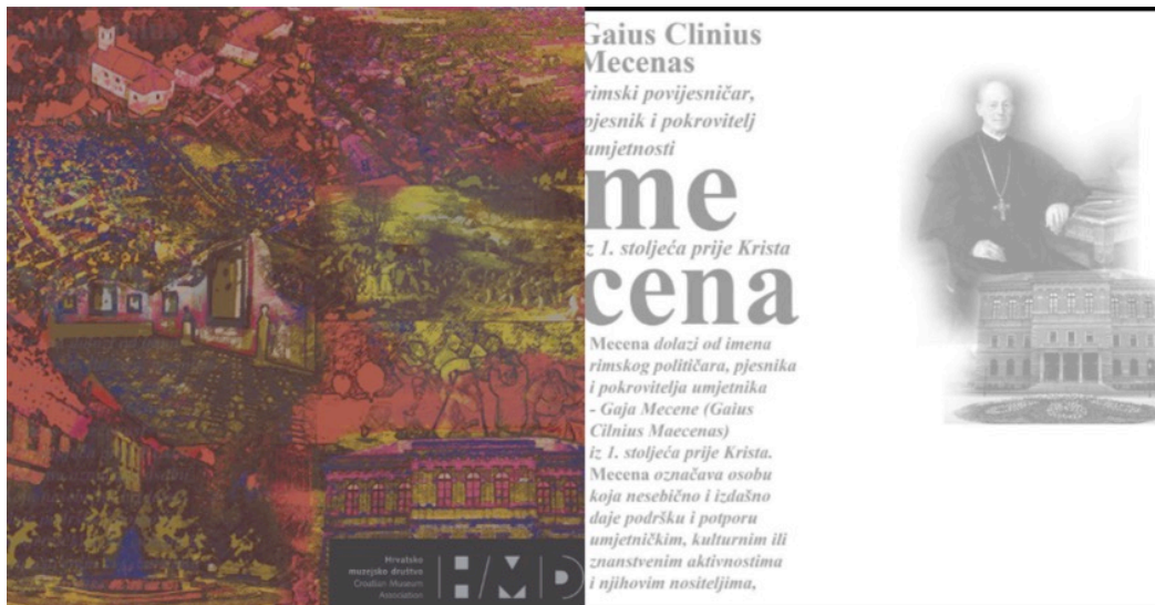
Figure 23. Dual graphic printed on textile in visual spectrum (left) and infrared (right)
