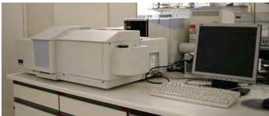
Figure 20: *Lambda 800 UV-VIS spectrophotometer.*
