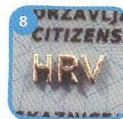
Taktilni element graviran laserom / Tactile element laser marked
