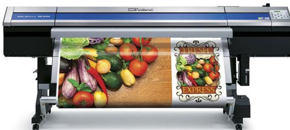
Slika 13-Prikaz digitalnog stroja Roland SOLJET Pro 4 XR-640 (izvor: http://mb.cision.com/Public/7229/9469538/846bd72139db5804_800x800ar.jpg )
