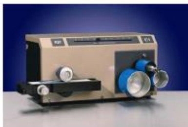
Slika 8. IGT Printability Tester C1 [21]
