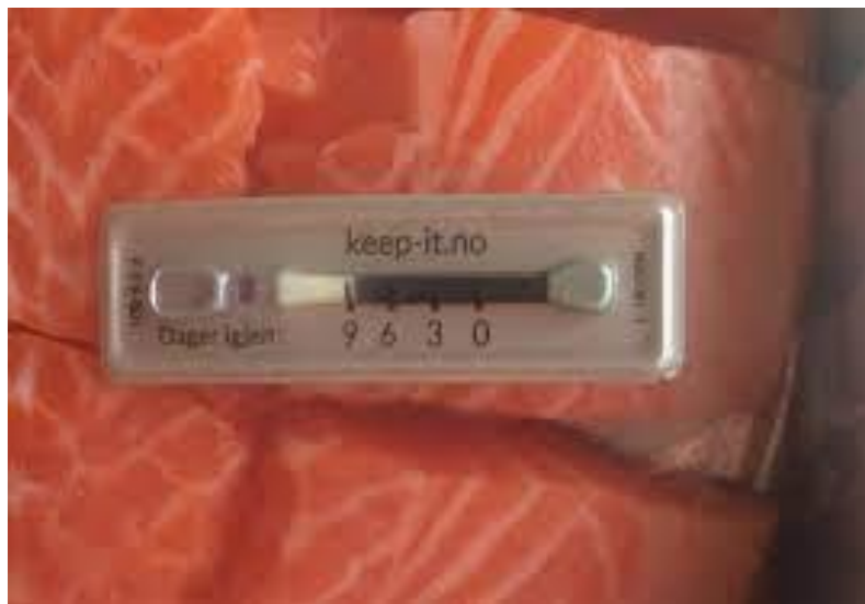
Slika 11.: Keep-It indikator vremena i temperature [8]
