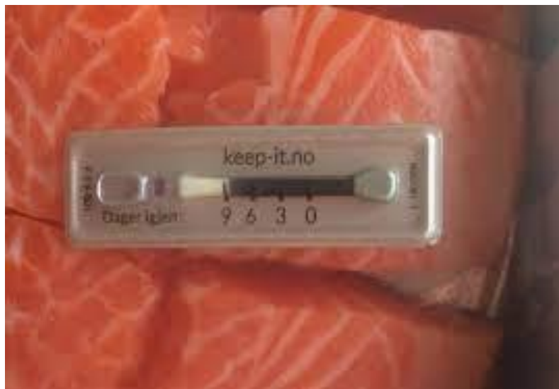
Slika 11.: Keep-It indikator vremena i temperature [8]
