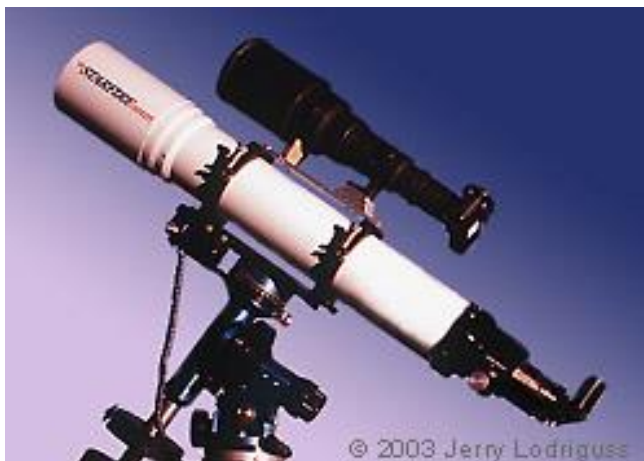
Slika 9. Piggyback metoda ( https://www.astropix.com/html/i_astrop/tracked/tracking.html )
