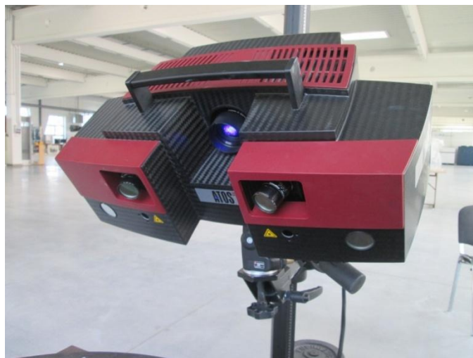
Figure 11: GOM ATOS II Rev. Scanner
