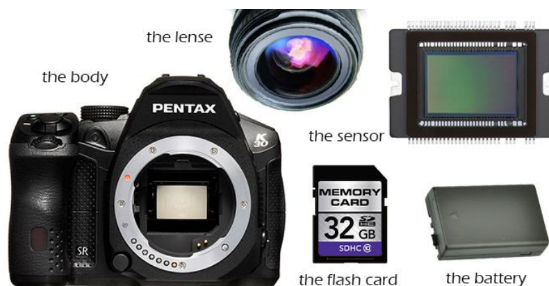
Image 1. Components of DSLR
