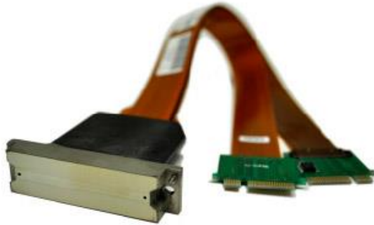
Slika 20. Ricoh Gen4 ispisna glava (Izvor: http://www.digiprint-supplies.com/en/ricoh-gen4-printhead-n220792-pphri12681.html )
