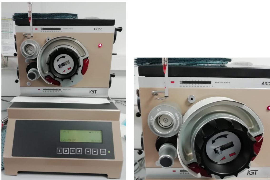
Figure 26 - IGT AIC2-5 in position for print penetration test
