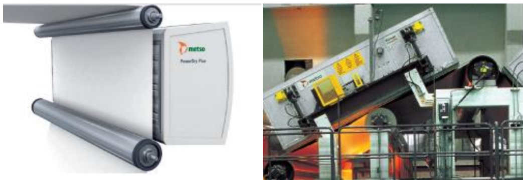
Figure 22- single-sided air impingement hood, left - web supported by rolls, right - web supported by nozzles
