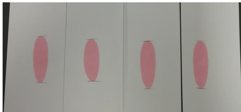
Figure 33 - Print penetration test on uncoated base paper
