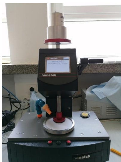
Slika 19. Hanatek Rub and Abrasion Tester
