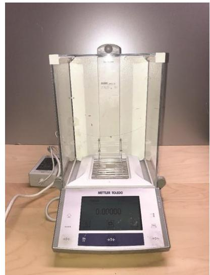
*Slika 15. Mettler Toledo XS205DU Dual Range Analytic Scale*
