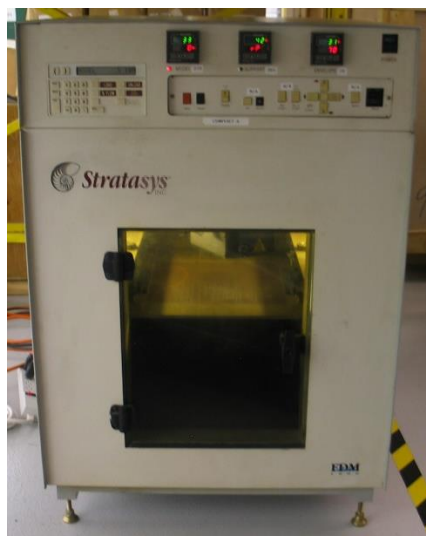
Slika 16. Stratasys FDM 1600 printer (Izvor: https://bit.ly/2wAekpO )
