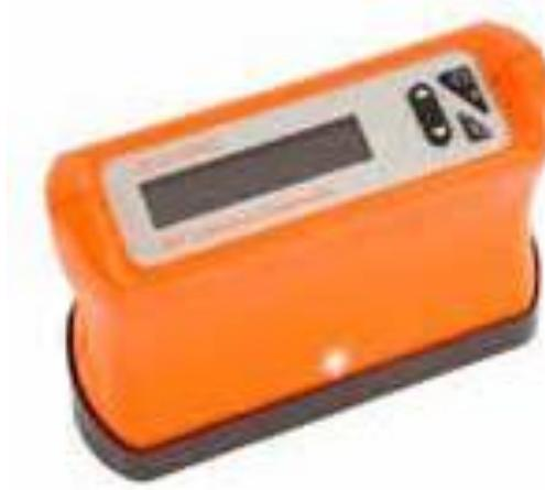
*Slika 38 Mjerni uređaj X-Rite Elcometer 407 Statistical Glossmeter (Izvor: [https://www.grf.unizg.hr/wp-content/uploads/2010/09/SMP\\_KatalogOpreme\\_FINAL-WEB\\_v2.pdf](https://www.grf.unizg.hr/wp-content/uploads/2010/09/SMP_KatalogOpreme_FINAL-WEB_v2.pdf))*
