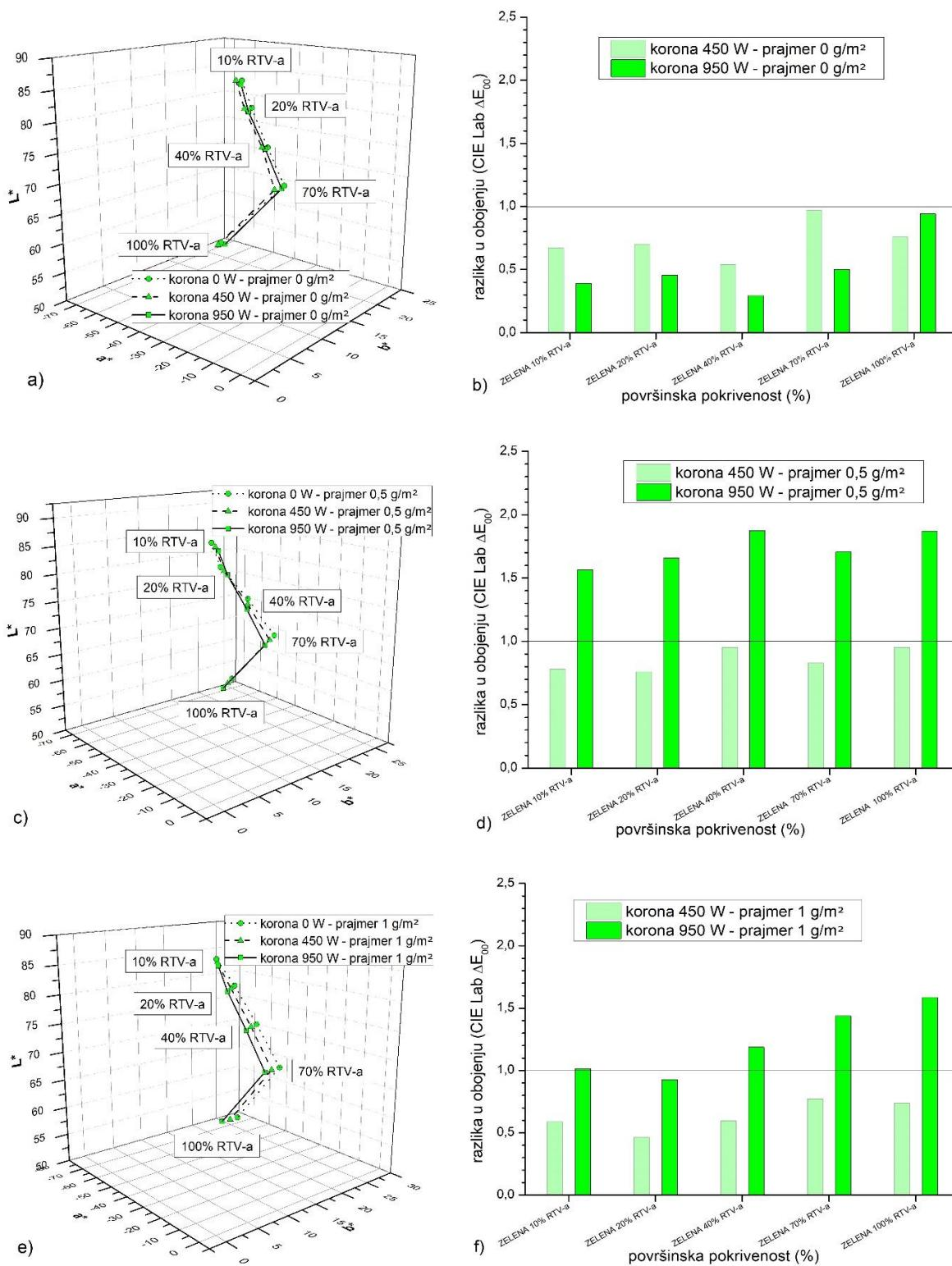
Slika 58. Zeleni otisci nakon varijacije korone: a) Lab bez prajmera; b)  $\Delta E$  bez prajmera; c) Lab  $0,5 \text{ g/m}^2$  prajmera; d)  $\Delta E 0,5 \text{ g/m}^2$  prajmera; e) Lab  $1 \text{ g/m}^2$  prajmera; f)  $\Delta E 1 \text{ g/m}^2$  prajmera
