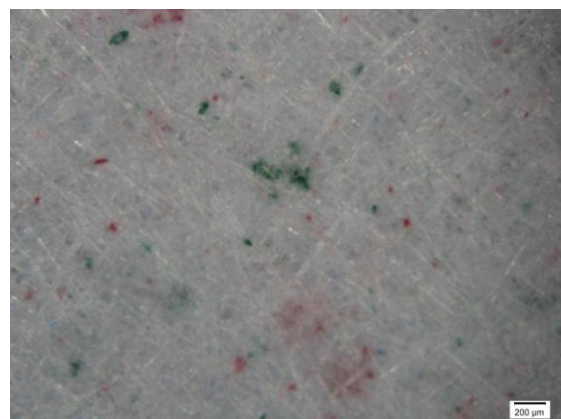
Fig 8 - Microscopic image of deinked pulp (DP) handsheet
