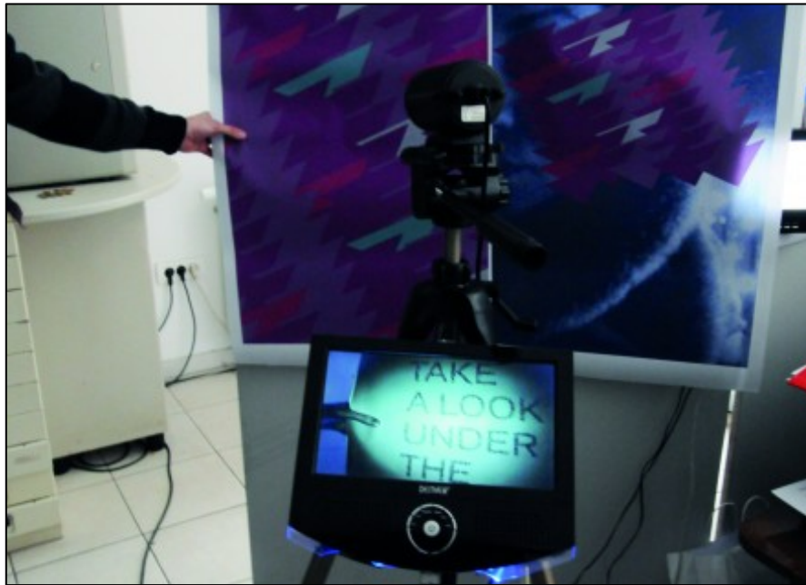
Figure 22. Usage of infrared camera to detect Z double information to design posters
