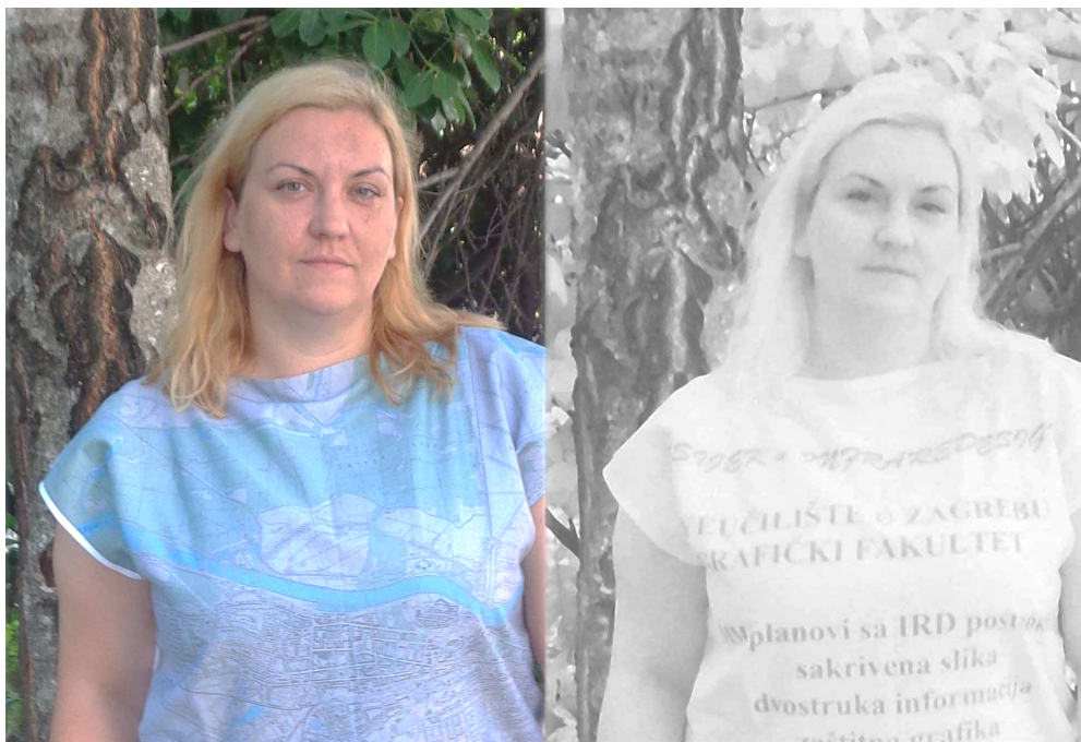
Figure 88. Clothing item designed with double imaging in the V and NIR spectrum
