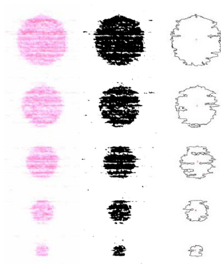
Figure 108. Original scan, binarized mask and outlines of the analyzed elements from test plate 7
