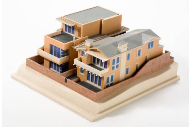
Figure 3. Example of a 3D colour print, model of a house, ©ZCorporation
