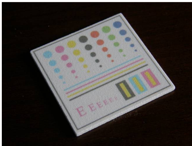
Figure 27. Example of printed and post-processed test plate
