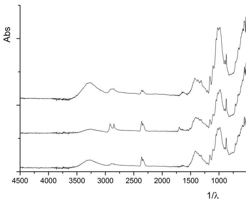
Slika 53. Od vrha prema dnu: FTIR spektri navigatorsa  $80\text{ g/m}^2$ , splendorgela  $115\text{ g/m}^2$ , arcoprinta  $120\text{ g/m}^2$
