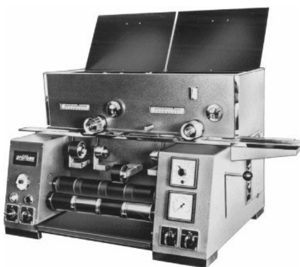
Slika 6. Uređaj Prufbau Multipurpose Printability Testing System
