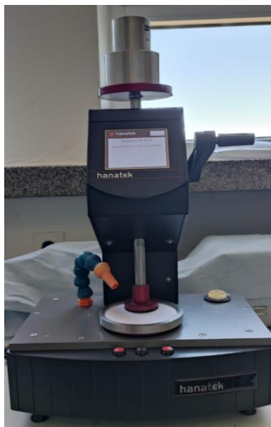
Slika 21. Hanatek Rub and Abrasion Tester
