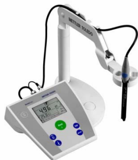
Slika 32 - pH metar Mettler Toledo SevenEasy 20S
