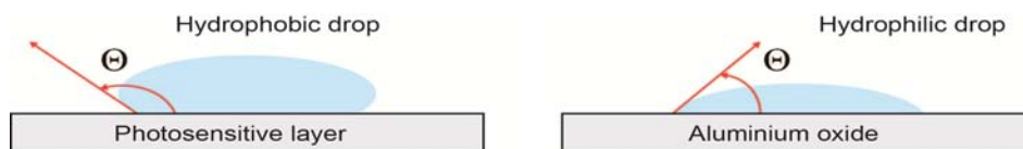
Figure 14. Relation between photosensitive layer and aluminium oxide with fountain solution drop
