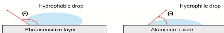
Figure 14. Relation between photosensitive layer and aluminium oxide with fountain solution drop
