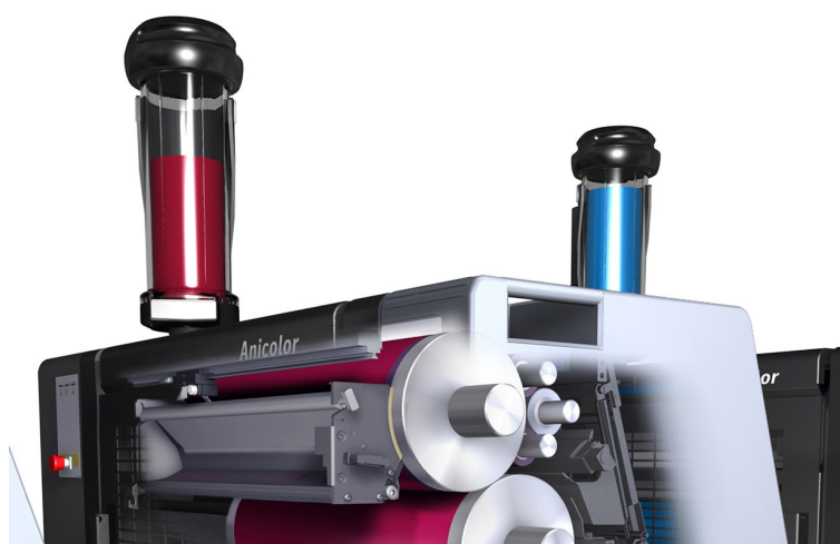
Slika 5. Handy Fill automatska opskrba bojom (Izvor: http://www.heidelberg.com/www/html/en/binaries/images/image_library/products/sheetfed/speedmaster_sm_52/071115_anicolor2 )
