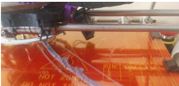
Figure 48: Building of support structure
