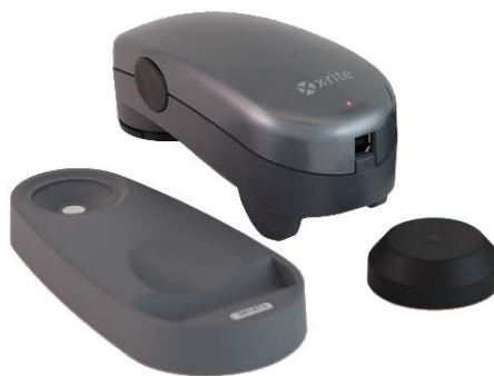
Slika 15 Spektrofotometar X-Rite i1 Pro ( http://www.tftcentral.co.uk/images/i1_pro/4.jpg )
