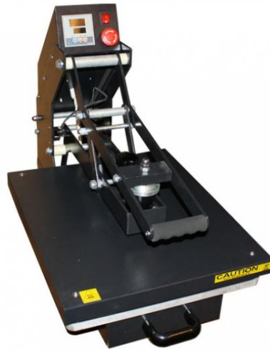
Slika 14 Termo preša DIPA MG-3 ( http://www.digitalpartner.hr/images/content/termo-prese/mg.jpg )
