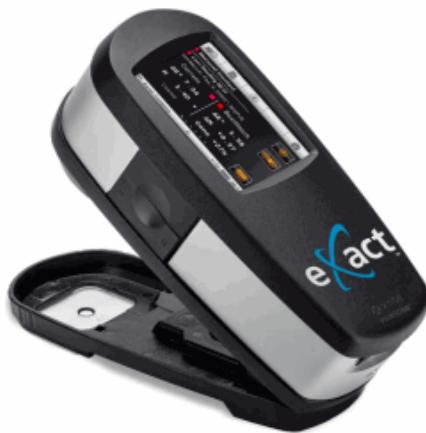
Slika 22. Spektrofotometar x-Rite Exact (Izvor: <http://www.flexodepot.com/X-Rite-eXact-P617.aspx>)
