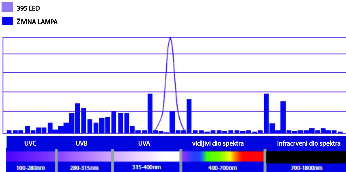
Slika 12. Usporedba valnih duljina živine žarulje i LED žarulje (Izvor: [http://uvledcommunity.org/uploads/pdfs/Technote-UV-LED-print-guide-US\\_web.pdf](http://uvledcommunity.org/uploads/pdfs/Technote-UV-LED-print-guide-US_web.pdf))
