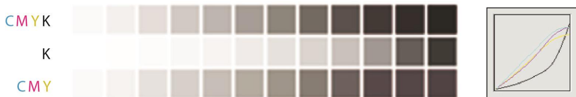
Slika 8. Postepeni rast crne Izvor: Homann, J-P. (2009). Digital Color Management Principles and Strategies for the Standardized Print Production
