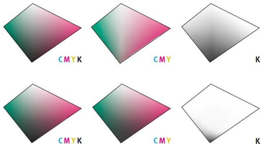
Slika 6. UCR i UCA Izvor: Homann, J-P. (2009). Digital Color Management Principles and Strategies for the Standardized Print Production
