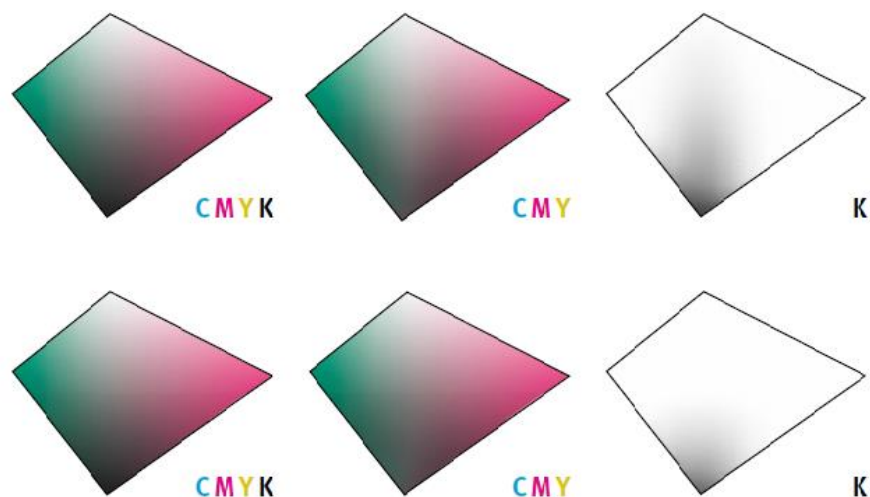
Slika 4. Duga i kratka crna Izvor: Homann, J-P. (2009). Digital Color Management Principles and Strategies for the Standardized Print Production
