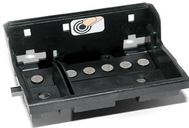
Slika 8. Ispisna glava za termalni Inkjet Kodak ESP (Izvor: http://www.kodak.com/us/en/consumer/products/printing-supplies/printhead-replacements/10-series-printhead/default.htm )
