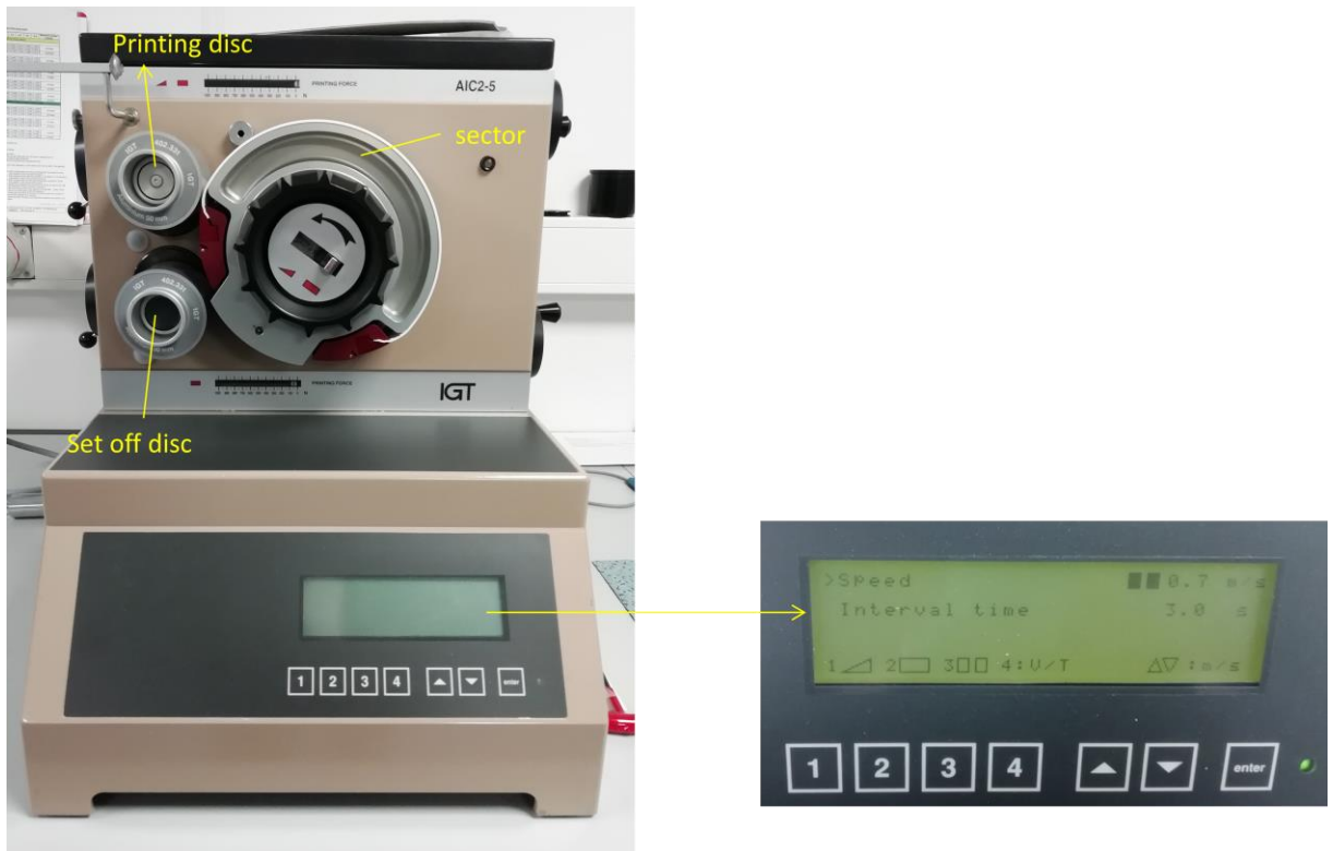
Figure 27 - IGT AIC2-5 in position for set off test
