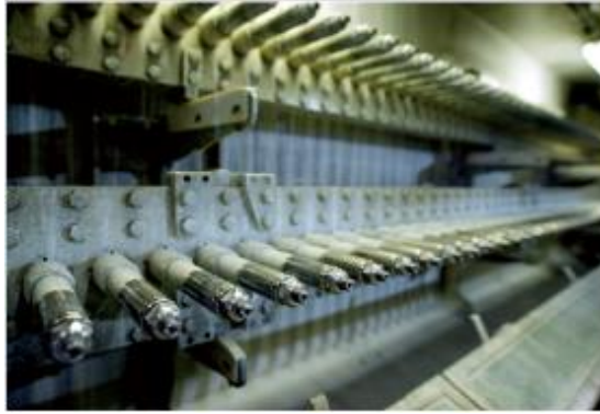
Figure 9– Spray nozzles in the coater
