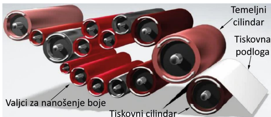
Slika 10. Shematski prikaz jedne letterpress jedinice [Flint Group Narrow Web, Inks, Coatings & Varnishes Workshop, brošura, 2017.]
