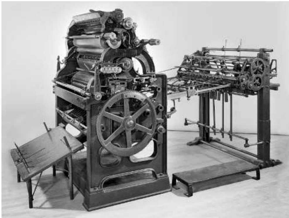
Slika 2. Komercijalni ofsetni sustav ( https://www.si.edu/es/object/nmah_882246 )
