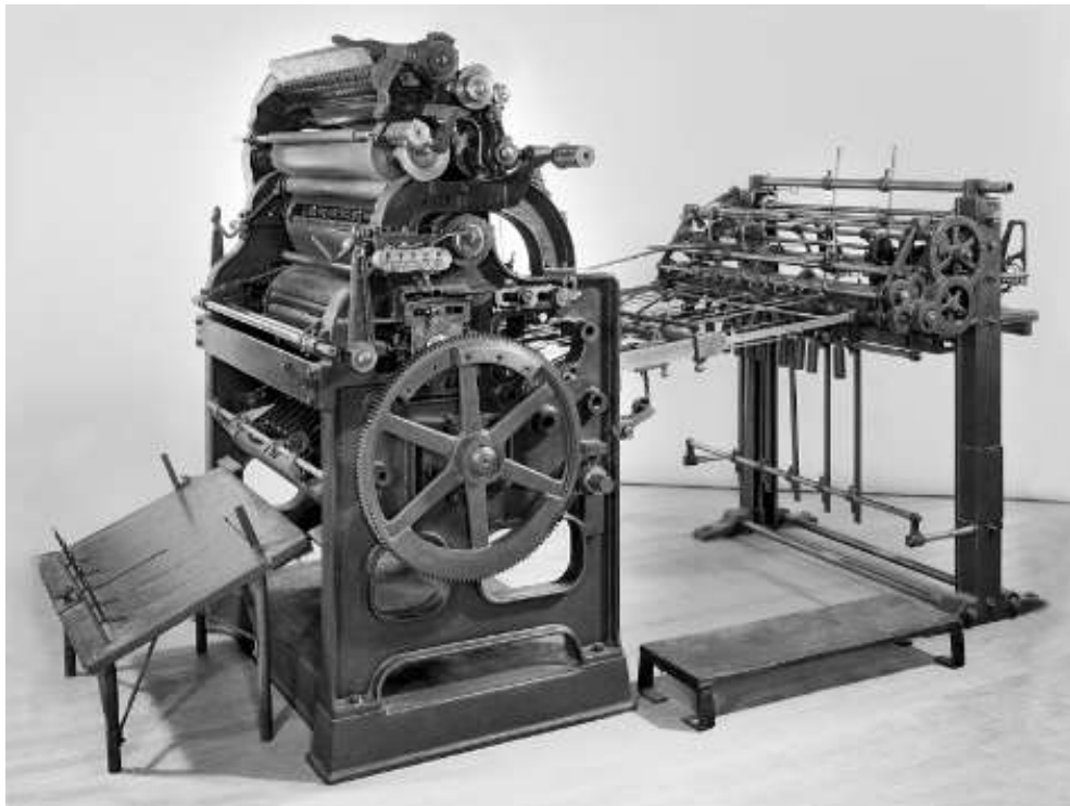
Slika 2. Komercijalni ofsetni sustav ( https://www.si.edu/es/object/nmah_882246 )
