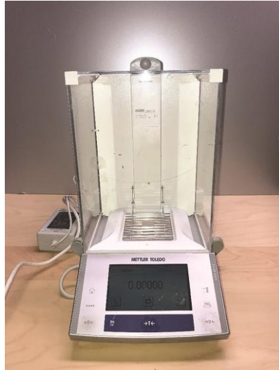
Slika 15. Mettler Toledo XS205DU Dual Range Analytic Scale
