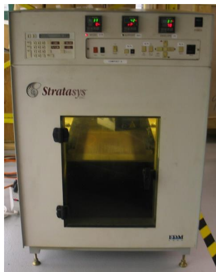
Slika 16. Stratasys FDM 1600 printer (Izvor: https://bit.ly/2wAekpO )
