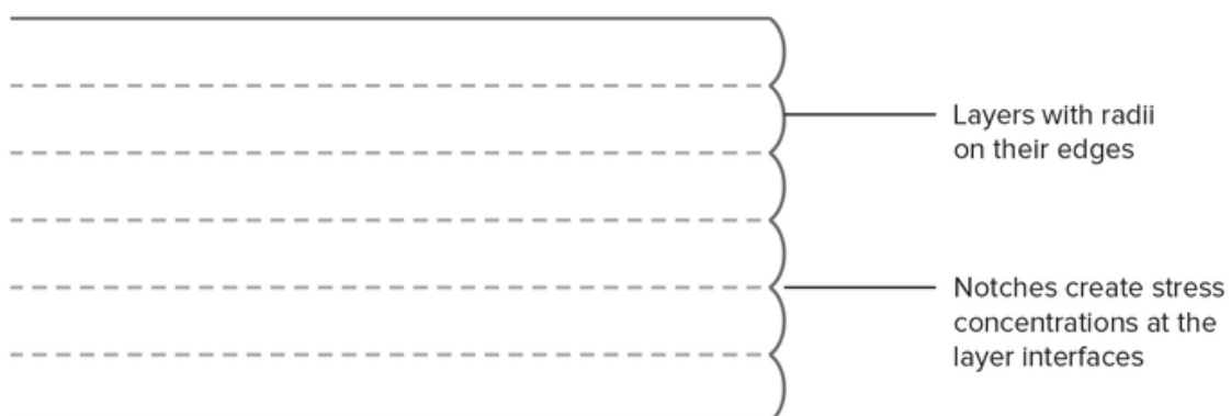
Slika 1.4 – Prikaz oblika FFF objekta ( https://www.3dhubs.com/knowledge-base/introduction-fdm-3d-printing )
