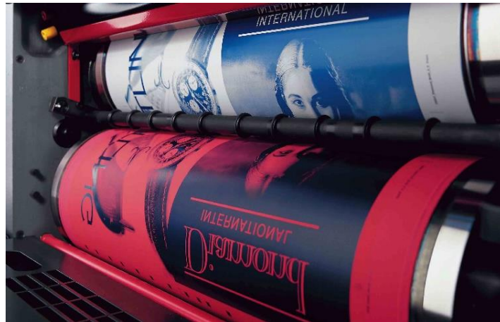
Figure 5 Offset printing process (plate to rubber (red) image transfer) [71]
