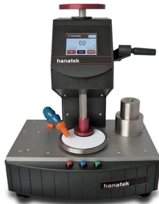
Figure 18 Hanatek RT4 Rub and Abrasion tester [116]
