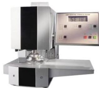
Figure 24 Lorentzen&Wettre Bursting Strength Tester [128]
