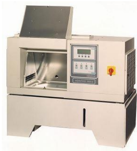
Figure 12 Solarbox 1500 e chamber [111]
