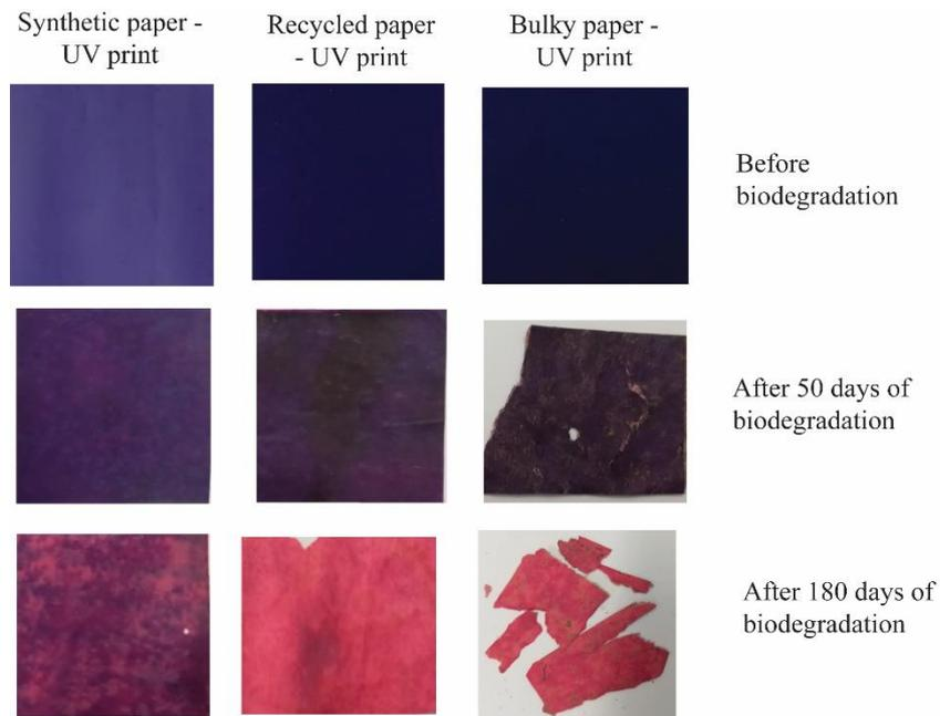
Fig 10. Visual evaluation of prints before and after 50 and 180 days of biodegradation
