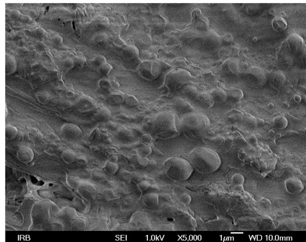
**Figure 23.** SEM micrograph of printed thermochromic offset ink on 33 % recycled paper after 150 days of biodegradation
