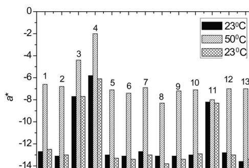
» **Figure 9:**  $a^*$  values of the prints at temperatures 23, 50 and repeated cooling to 23 °C (1-original and after interaction with: 2- benzene, 3-acetone, 4-cyclohexanone, 5-propan-2-ol, 6-isobutanol, 8-pentanol, 9-hexanol, 10-cyclohexanol, 11-ethanol, 12-ethylene glycol, 13-water)
