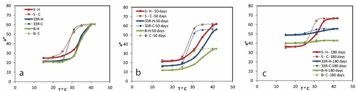
**Figure 44.** CIELAB  $a^*$  values of UV print on synthetic paper ( S - red), recycled paper (33R - blue) and bulky paper (B - green) in dependence on temperature at heating (solid line) and cooling (open line) before biodegradation (a), after 50 days of biodegradation (b) and after 180 days of biodegradation (c).
