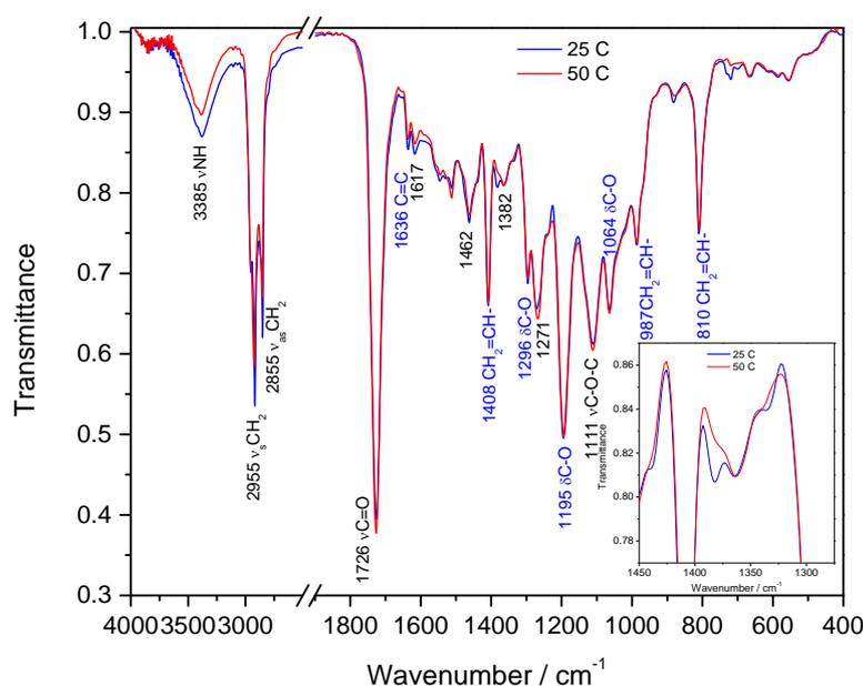
**Figure 27.** FTIR spectra of the UV curable screen printing thermochromic ink at 25 °C and 50 °C, measured in transmission mode
