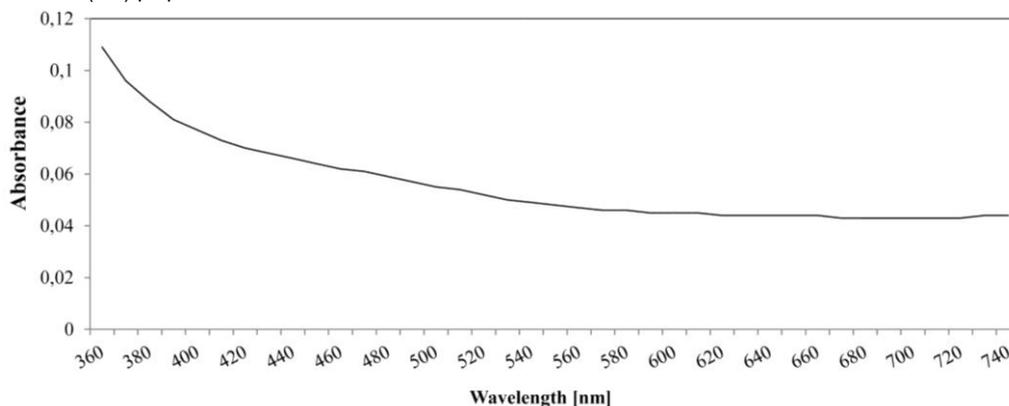
Fig 12 - Absorbance spectra of froth filtrate
