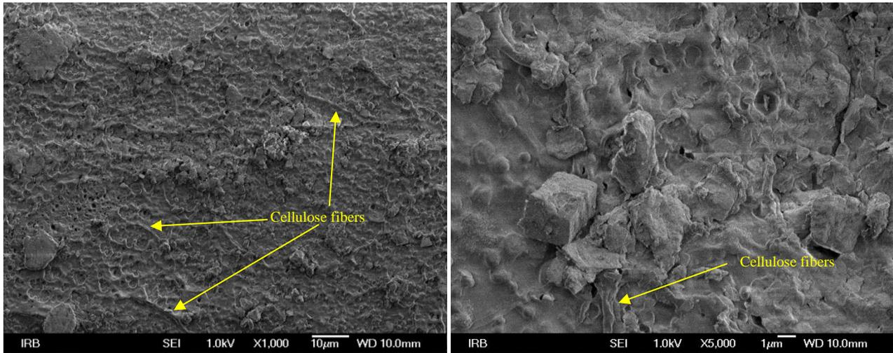
Fig 9. SEM micrograph of UV print on bulky paper after 180 days of biodegradation under different magnifications (1000x and 5000x)
