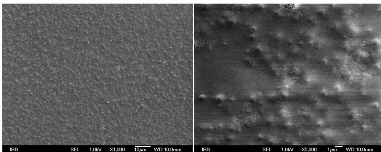
Fig 4. SEM micrograph of UV print on synthetic paper before biodegradation under different magnifications (1000x and 5000x)
