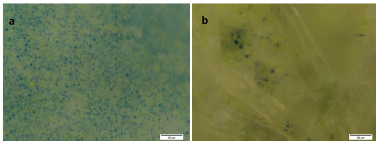
Fig 12 - Microscopic image of thermochromic prints on synthetic (a) and recycled paper (b) after 150 days of biodegradation.
