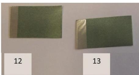
» **Figure 4c:** Thermochromic print after interaction with: 12-ethylene glycol, 13-distilled water
