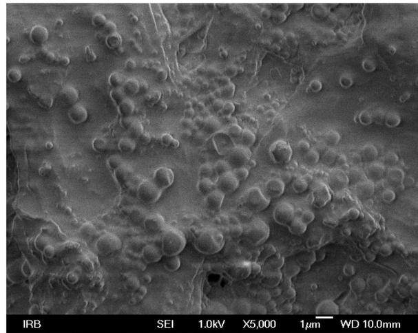
Fig 4 - SEM micrograph of printed thermochromic ink on recycled paper before biodegradation.
