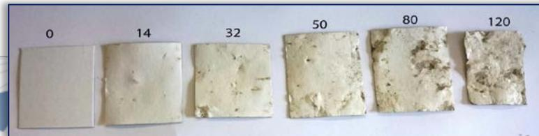
Figure 3: Biodegradation over 120 days for neat UC cardboard
