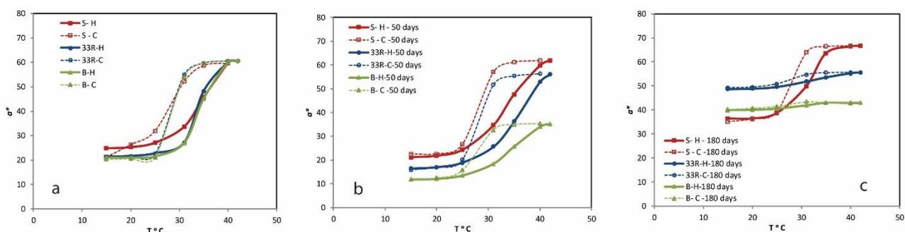
Fig 20. *CIELAB a\** values of UV print on synthetic paper (S - red), recycled paper (33R - blue) and bulky paper (B - green) in dependence on temperature at heating (solid line) and cooling (open line) before biodegradation (a), after 50 days of biodegradation (b) and after 180 days of biodegradation (c).
