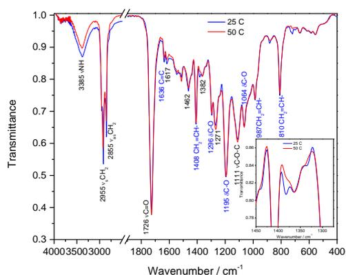
Fig 1. FTIR spectra of the UV thermochromic ink at 25 °C and 50 °C, measured in transmission mode
