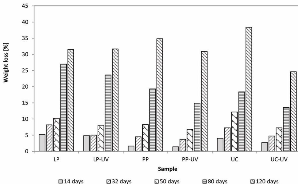
**Figure 48.** Biodegradation of samples through weight loss over 120 days
