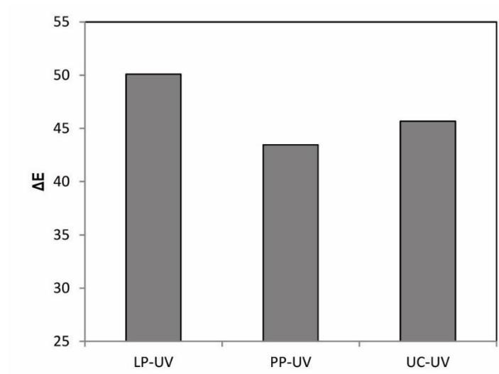
**Figure 49.** Total colour difference after 120 days of biodegradation
