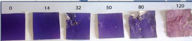
Figure 4: Biodegradation over 120 days for printed LP - UV cardboard
