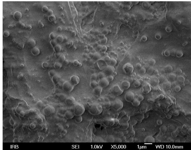
**Figure 22.** SEM micrograph of printed thermochromic offset ink on 33% recycled paper before biodegradation
