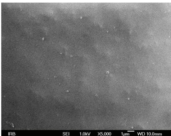
» **Figure 5:** SEM micrograph of original green thermochromic print (magnification 5000x)
