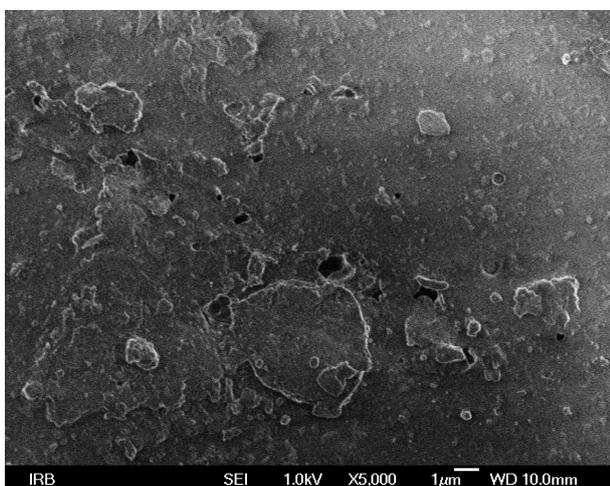
Fig 3 - SEM micrograph of printed thermochromic ink on synthetic paper after 150 days of biodegradation.
