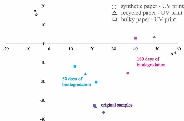
**Figure 41.** Colorimetric properties ( $a^*$  and  $b^*$  values) of UV prints measured at 20°C before (purple), after 50 days (blue) and 180 days (pink) of biodegradation (circle- UV print on synthetic paper, triangle – UV print on recycled paper, square – UV print on bulky paper)
