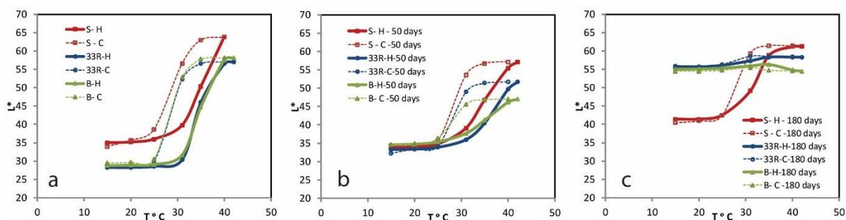
**Figure 42.** CIELAB  $L^*$  values of UV print on synthetic paper (S - red), recycled paper (33R - blue) and bulky paper (B - green) in dependence on temperature at heating (solid line) and cooling (open line) before biodegradation (a), after 50 days of biodegradation (b) and after 180 days of biodegradation (c).
