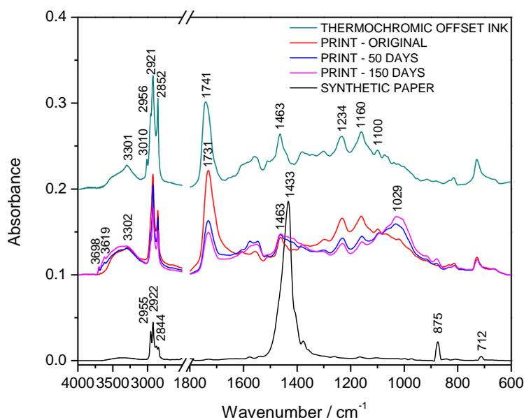
**Figure 24.** FTIR spectra of the thermochromic offset ink, neat S paper and prints of thermochromic offset ink on S paper before and after 50 and 150 days of biodegradation
