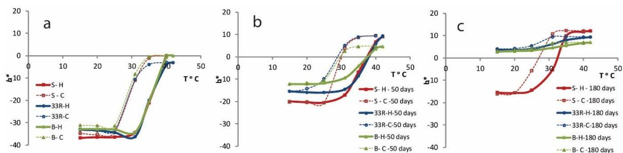
**Figure 43.** CIELAB  $b^*$  values of UV print on synthetic paper (S - red), recycled paper (33R - blue) and bulky paper (B - green) in dependence on temperature at heating (solid line) and cooling (open line) before biodegradation (a), after 50 days of biodegradation (b) and after 180 days of biodegradation (c).
