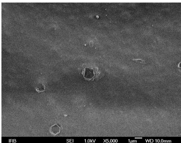
Fig 2 - SEM micrograph of printed thermochromic ink on synthetic paper before biodegradation.
