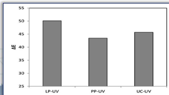
Figure 11: Total colour difference after 120 days of biodegradation
