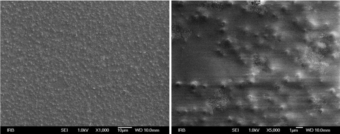
**Figure 29.** SEM micrograph of UV print on synthetic paper before biodegradation at different magnifications (1000x and 5000x)
