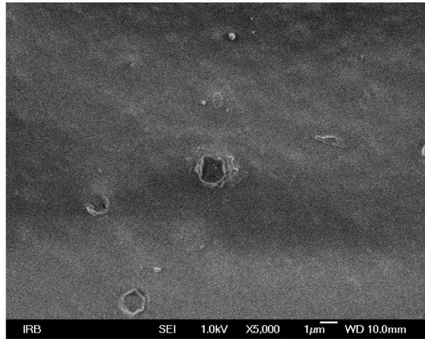
**Figure 20.** SEM micrograph of printed thermochromic offset ink on synthetic paper before biodegradation
