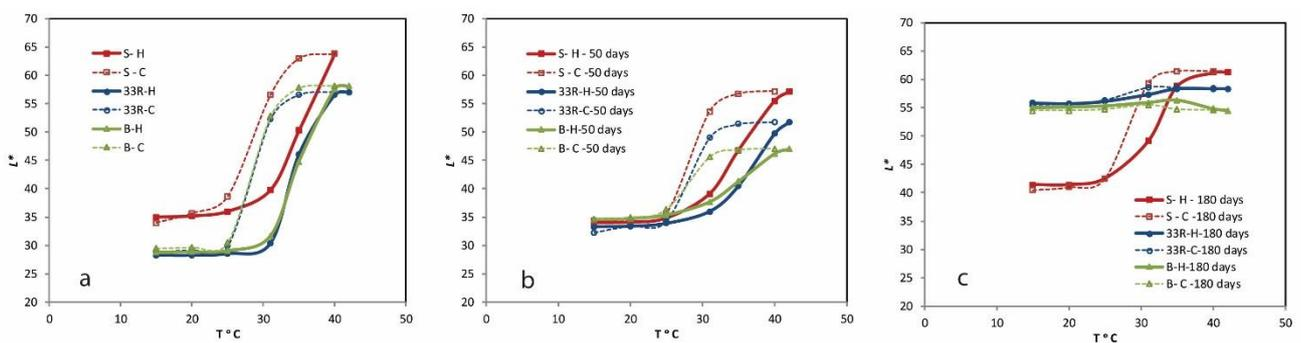
Fig 18. CIELAB  $L^*$  values of UV print on synthetic paper (S - red), recycled paper (33R - blue) and bulky paper (B - green) in dependence on temperature at heating (solid line) and cooling (open line) before biodegradation (a), after 50 days of biodegradation (b) and after 180 days of biodegradation (c).
