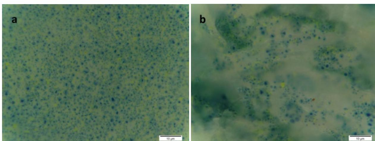
Fig 11 - Microscopic image of thermochromic prints on synthetic (a) and recycled paper (b) after 50 days of biodegradation.
