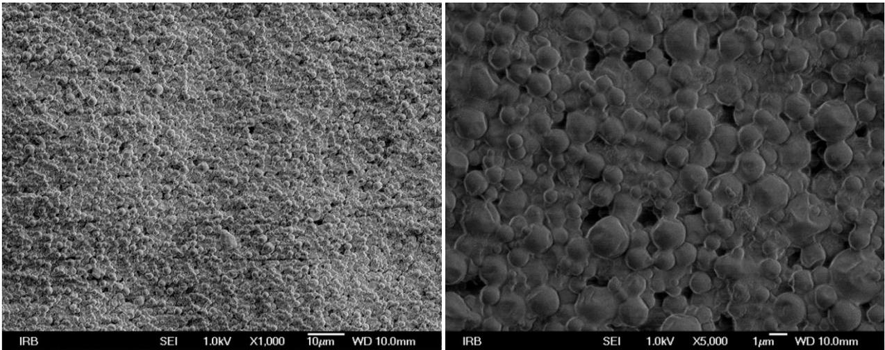
Fig 8. SEM micrograph of UV print on bulky paper before biodegradation under different magnifications (1000x and 5000x)
