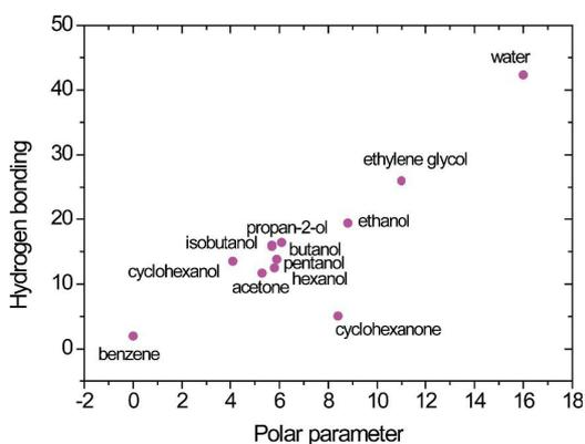
» **Figure 12:** Relation between hydrogen bonding and polar parameters of tested solvents
