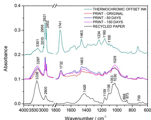
Fig 8 - FTIR spectra of the thermochromic ink, neat recycled paper and prints of thermochromic ink on recycled paper before and after 50 and 150 days of biodegradation.
