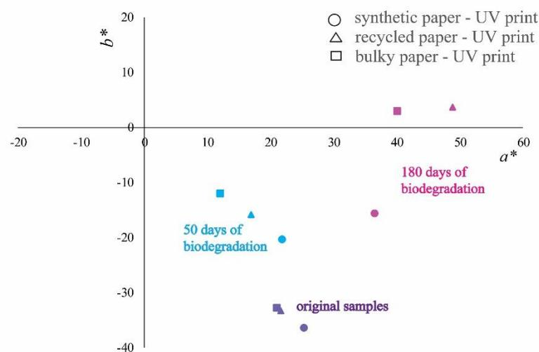
Fig. 17. Colorimetric properties ( $a^*$  and  $b^*$  values) of UV prints measured at 20°C before (purple), after 50 days (blue) and 180 days (pink) of biodegradation (circle- UV print on synthetic paper, triangle – UV print on recycled paper, square – UV print on bulky paper)
