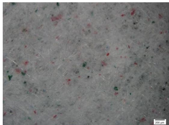
Fig 7 - Microscopic image of undeinked pulp (UP) handsheet
