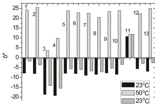
» **Figure 10:**  $b^*$  values of the prints at temperatures 23, 50 and repeated cooling to 23 °C (1-original and after interaction with: 2- benzene, 3-acetone, 4-cyclohexanone, 5-propan-2-ol, 6-isobutanol, 7-pentanol, 8-hexanol, 9-cyclohexanol, 10-cyclohexanol, 11-ethanol, 12-ethylene glycol, 13-water)
