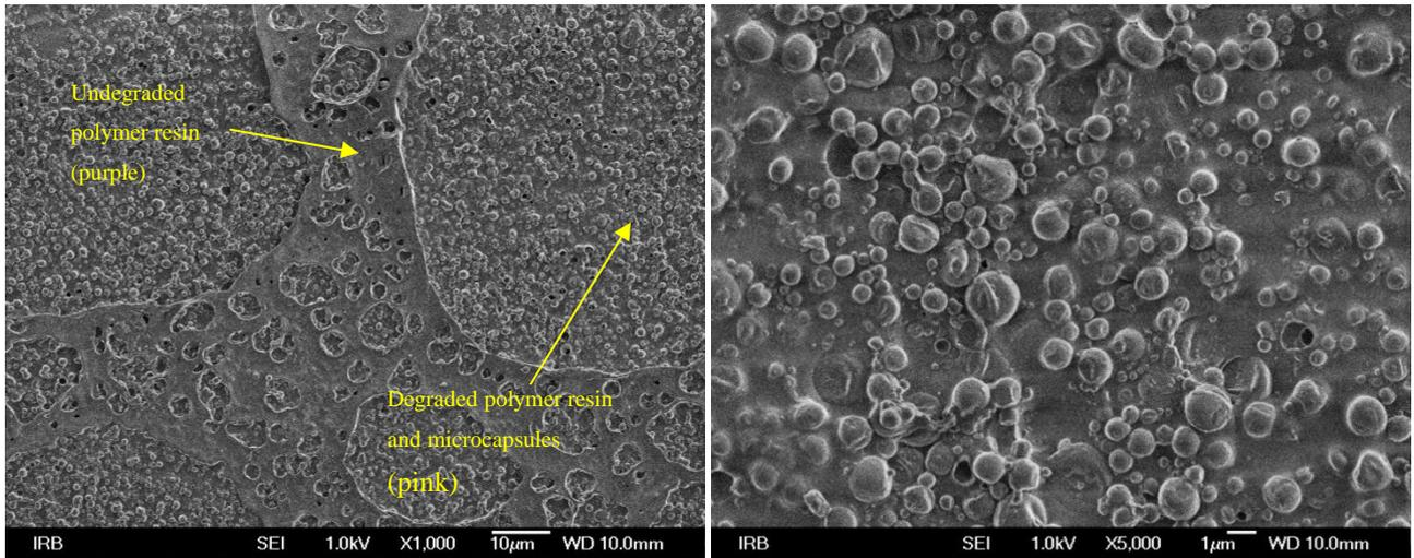
Fig 5. SEM micrograph of UV print on synthetic paper after 180 days of biodegradation under different magnifications (1000x and 5000x)
