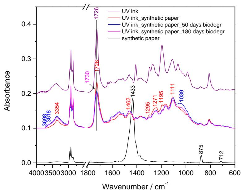
**Figure 38.** FTIR spectra of the UV thermochromic ink, the neat synthetic paper and the prints of the ink on the synthetic paper before and after 50 and 180 days of biodegradation, measured in ATR mode
