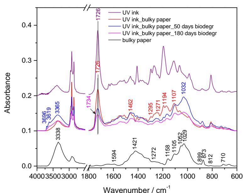
**Figure 40.** FTIR spectra of the thermochromic ink, the neat bulky paper and the prints of the ink on the bulky paper before and after 50 and 180 days of biodegradation, measured in ATR mode.
