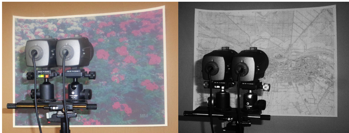
Figure 30. NIR camera with dual option of V and Z recording
